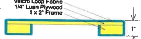
Panel With Interior Frame
